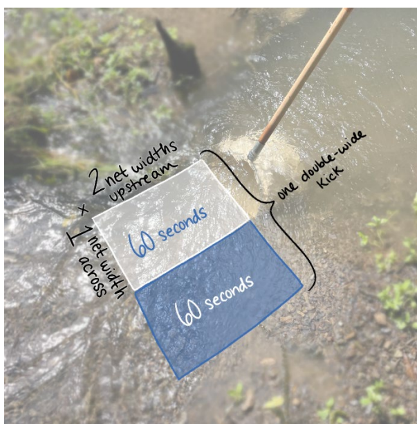
Figure 33: For a double-wide kick, after a location is monitored, place the net directly adjacent to the location and begin again.
