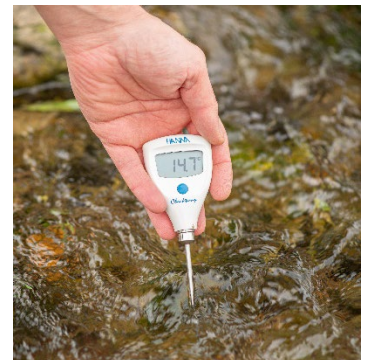
Figure 6: Water Temperature reading.
