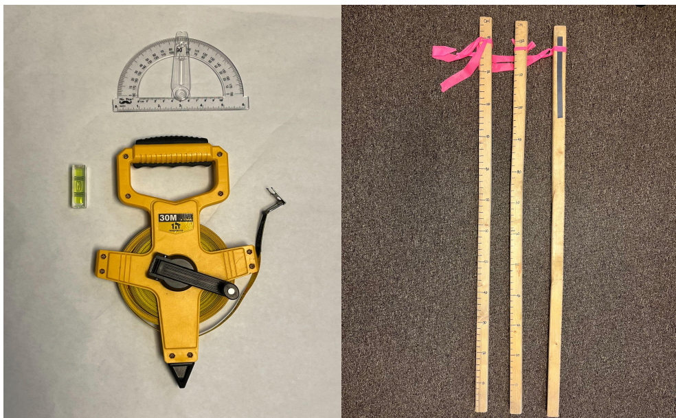
Figure 7. Gage sticks, protractor, and measuring tape. Photo credit: Alliance
