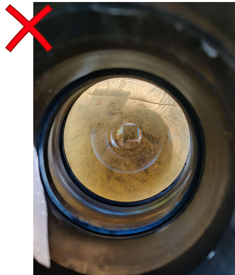
Figure 21. Example of a bad stream viewer photo. Photo has a strong reflection, is not clear and does not cover the entire stream viewer. Photo credit: Alliance
